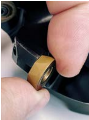
① Position the indexable insert
