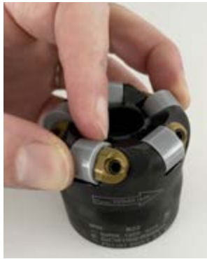
② Fit the ceramic indexable insert
