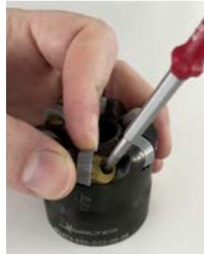
③ Secure the ceramic indexable insert
