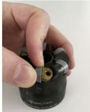
② Fit the ceramic indexable insert
