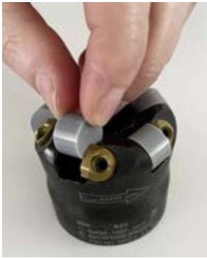
① Insert the ceramic indexable insert
