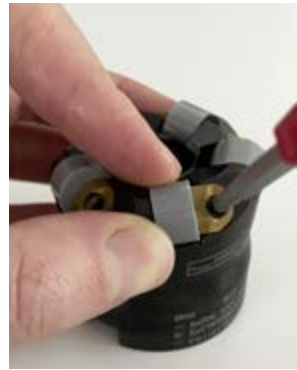
③ Secure the ceramic indexable insert
