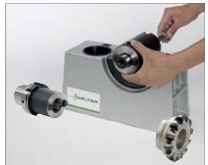
6. Screw the extension and the end mill adaptor together by hand using the socket wrench
