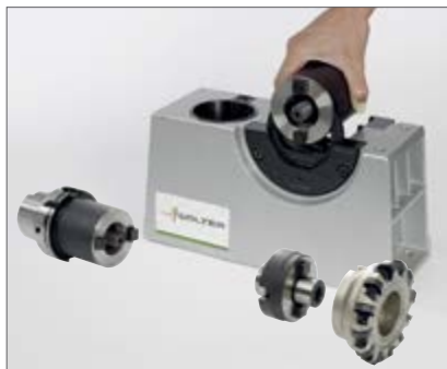
5. Insert the extension into the insert collar
