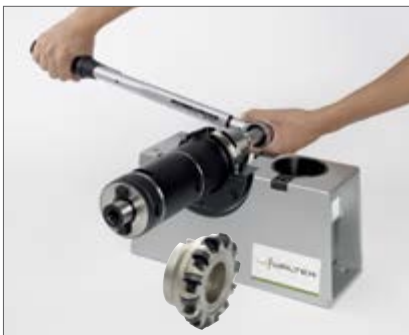
10. Tighten using a torque wrench
