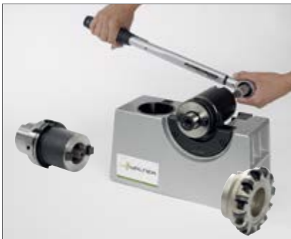
7. Tighten using a torque wrench
