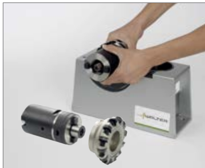
8. Insert the master into the associated flange
