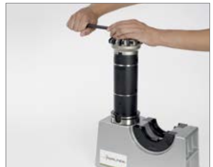
12. Install and tighten the tool
